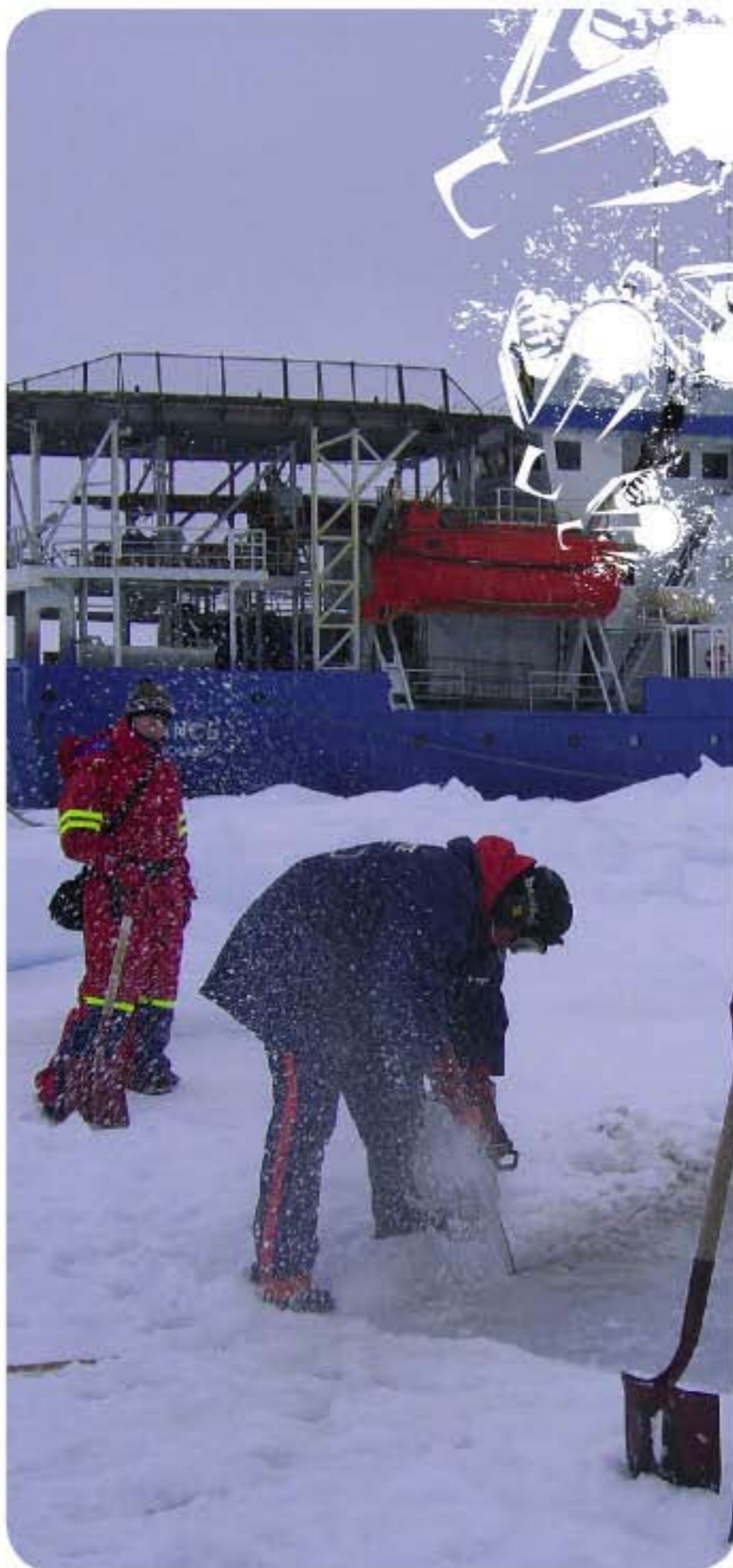
Oil spills in ice infested waters is a major research focus for the Technology department. Experiments with oil spills and remediation techniques are tested out in small areas on the ice, which requires digging out small pools in the sea ice. This image is from the Technology cruise with R/V "Lance" in May 2006.
