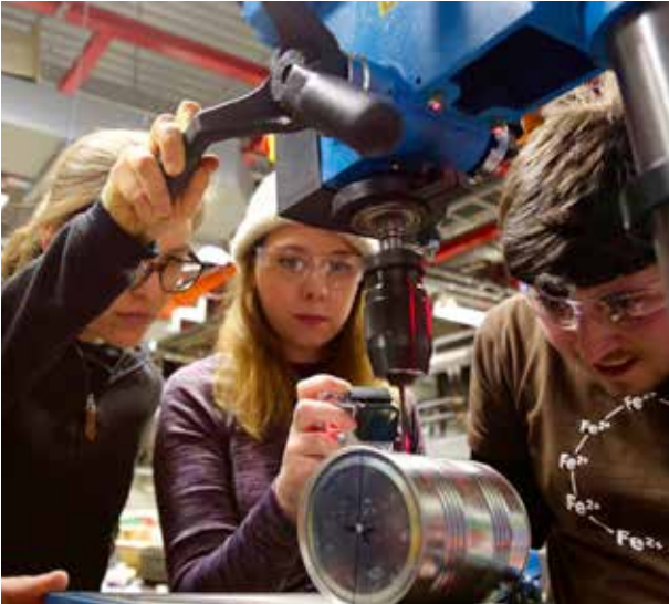
February 2017: AGF-304/804 Radar Diagnostics of Space Plasma students build "cantennas"; small antenna radars built out of old metal boxes. Photo: Anja Strømme/UNIS.
