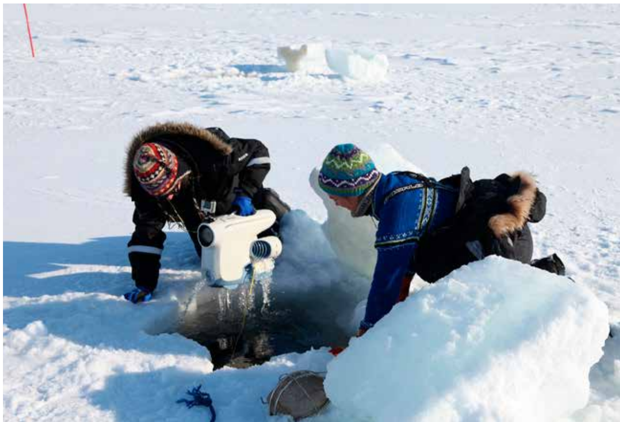
April 2017: The underwater drone «BluEye», developed by NTNU (AMOS), is tested in Van Mijenfjorden. Photo: Martin Ludvigsen/UNIS.
