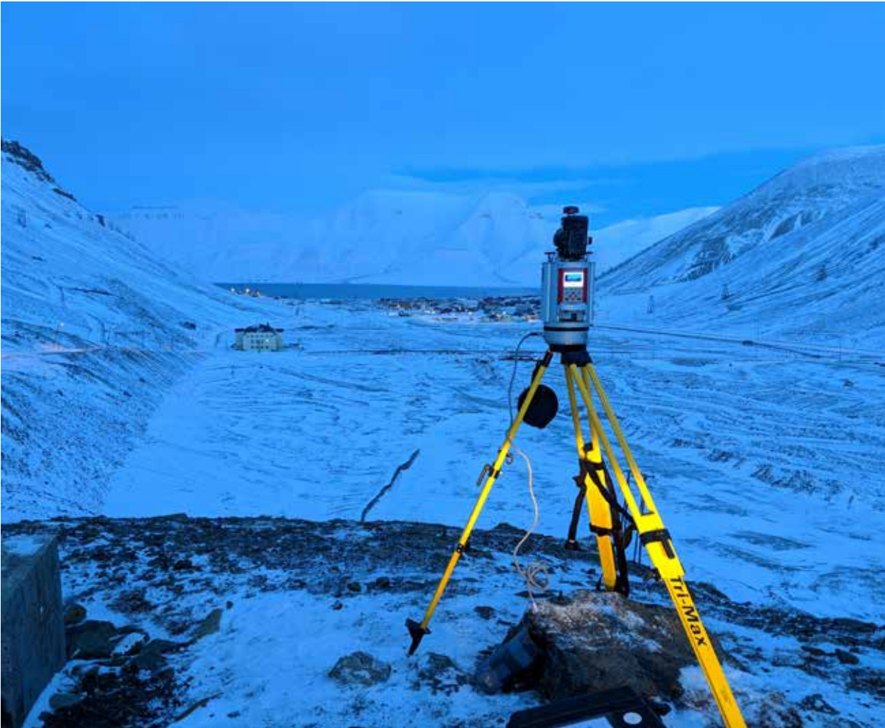
October 2019: The Arctic technology department perform laser scanning of the roads in Longyearbyen. Photo: Nataly Marchenko/UNIS.
